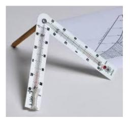
With those two values known, the other properties of the air, including its moisture content, can be determined by computation or by reading a <u>psychrometric chart.</u>
