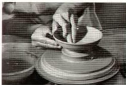
FIGURE 11. The bowl is thinned using a wooden shaper.
