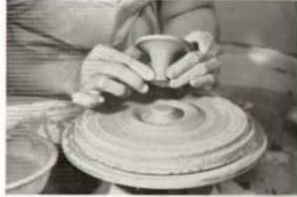
FIGURE 24. The foot is lifted from the wheel.
