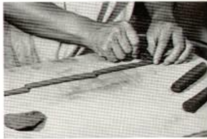
FIGURE 50. The clay is cut to equal lengths.
