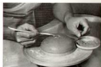
FIGURE 44. Wet clay is applied as a bowl.
