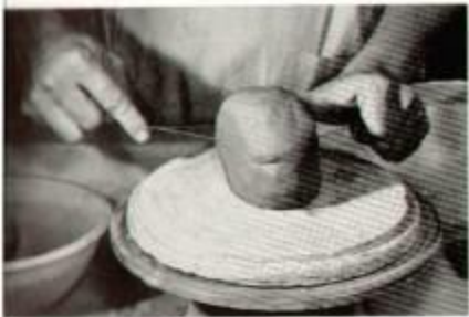
FIGURE 1. The clay is cut in half with a wire. (p. 9)
