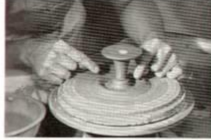
FIGURE 23. A wire is slowly drawn through the base.
