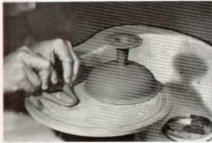
FIGURE 53. The ends are cut at an angle to fit the bowl.
