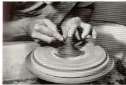
FIGURE 35. The foot is turned with a metal shaver.
