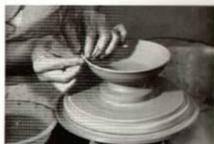
FIGURE 12. A wet leather strip finishes the lip.
