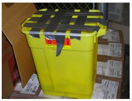
This container was refused by our biohazardous waste vendor because the container did not meet DOT transport regulations. Taping the top of the container allows for sharps or blood and bloody fluids to leak around the weave of the tape, if the container should tip over. Large biohazardous waste and chemo waste containers such as these must be sealed with a tightly fitting lid prior to transport.
