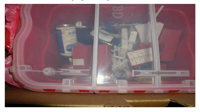
This red container was returned by the waste vendor, because it contains an aerosol can. Biohazardous waste undergoes both heat and pressure as part of the process that renders biohazardous waste non-infectious. Aerosol cans, even if empty, can act as a small bomb if placed under these conditions, creating a very unsafe condition for employees handling this waste. Aerosol cans must NEVER go in biohazardous waste. Aerosol cans are required by law to be recycled on our campus.
