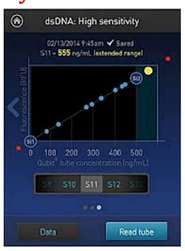
The Qubit® 2.0 Fluorometer displays the standard curve after completion of the calibration.
