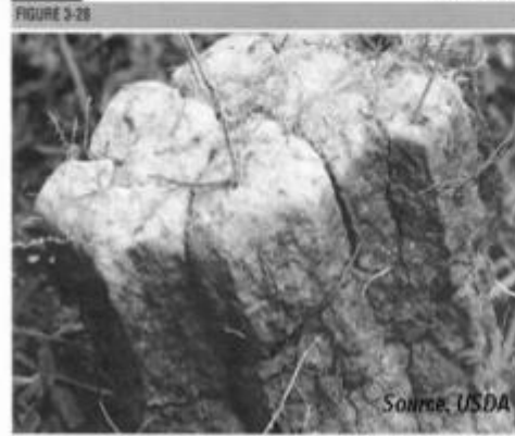
A cluster of strong medium-columnar peds. The cluster is about 125 mm across.
