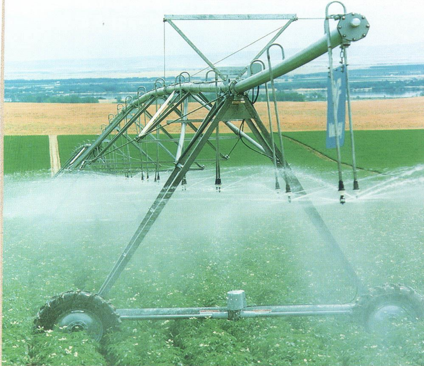
System shown with 80" (2.03 m) spacing, galvanized steel drops, pressure regulators and Valley spray nozzles.
