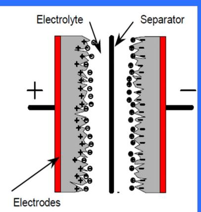
Figure 2: Supercapacitor sketch
