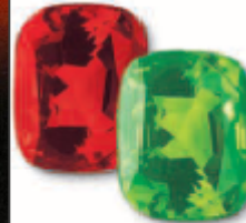
Color change Alexandrite exhibits color change—from brilliant green in daylight to cherry-red under tungsten light.
