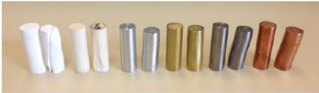
Fig. 2.3 Porous \text{Al}_2\text{O}_3 , Non-Porous \text{Al}_2\text{O}_3 , aluminum, brass, steel, copper. Each pair of materials contain samples before (left) and after (right) compression testing.
