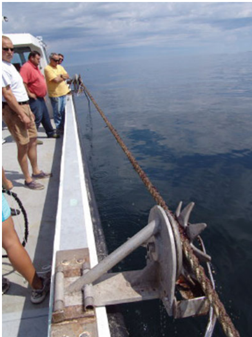
Mussel Culture, Open Ocean Innovations. Figure 3 A forward looking view of the starboard side of a service vessel showing the backbone of a submerged longline set into aft (foreground) and forward starwheels. Growing ropes with seed mussels are attached to the backbone for the growout cycle
