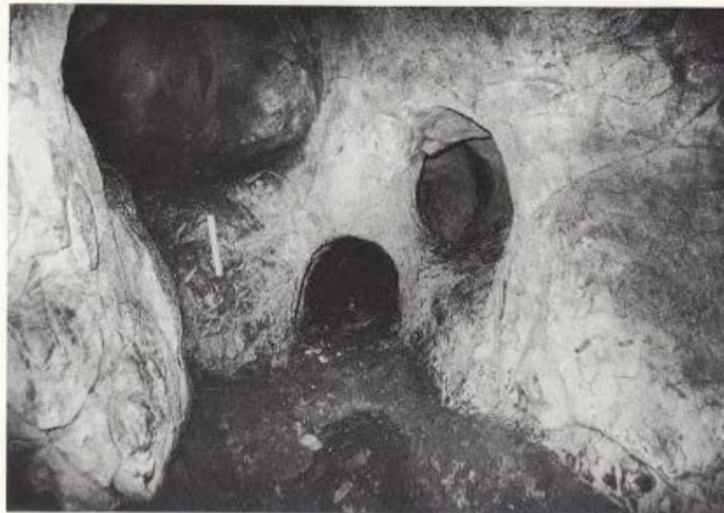
FIGURE 2.6 Complex fireset working at the Kestel tin mine dating from the third millennium BC. Note the smooth continuous contours of the walls, and the very precise nature of the work quite typical of fire-setting.
