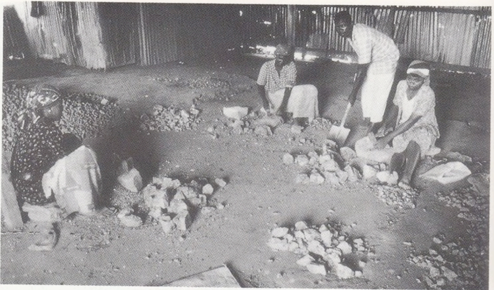
FIGURE 5.6 Hand crushing and sorting lead-zinc ores at Ishiagu, southern Nigeria, 1990. This was the traditional method of primary ore sorting until the recent past, and was usually performed by women and children.
