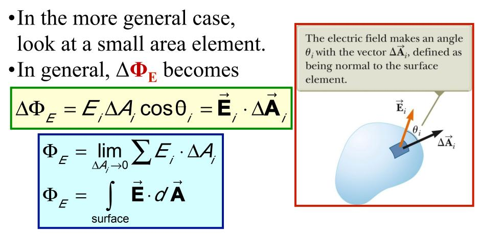
• The surface integral means that the integral must be evaluated over the surface in question. In general, the value of the flux will depend both on the field pattern & on the surface. • The Electric Flux  $\Phi_E$  through a <u>closed surface</u> is <u>defined</u> as the closed surface integral of the scalar (dot) product of
