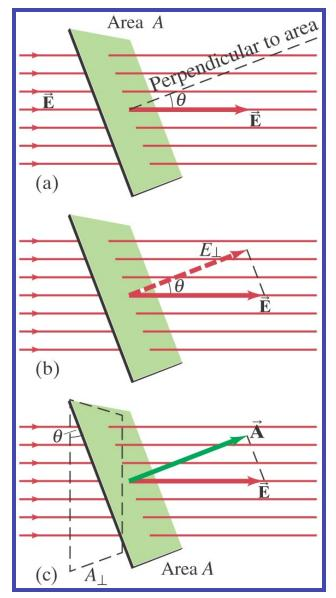
The Electric Flux Φ<sub>E</sub> through a cross sectional area A is proportional to the total number of field lines crossing the area & is
