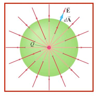
Using <u>Coulomb's Law</u> to evaluate the integral of the field of a point charge over the Surface of a sphere of surface area A<sub>1</sub> surrounding the charge gives:
