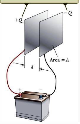
(a) A <u>Parallel-Plate Capacitor</u> connected to a battery.
