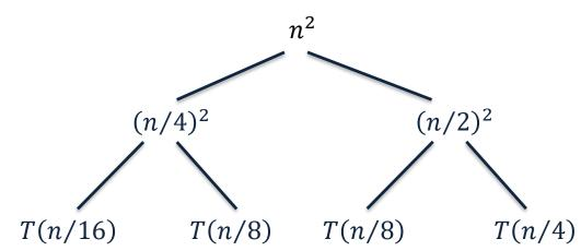
$$T(n) = \begin{cases} 1 & \text{,} & \text{if } n \le 1 \\ T(n/4) + T(n/2) + n^2 & \text{,} & \text{if } n > 1 \end{cases}$$
