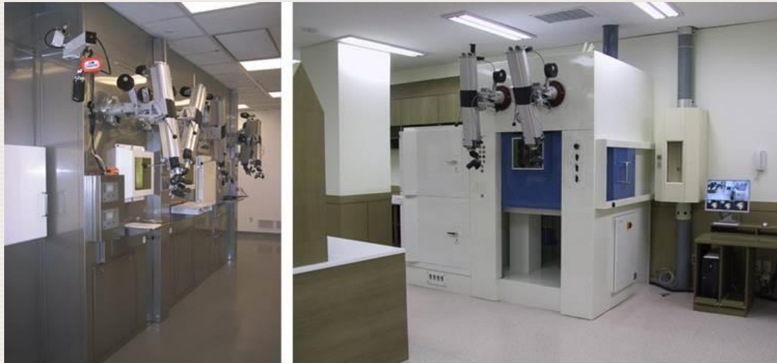
Examples of modern hot-box designs
