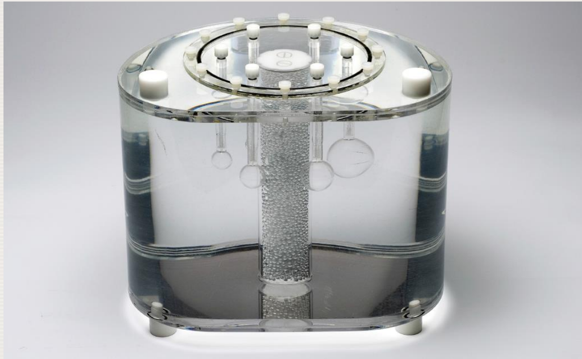
IEC/NEMA IQ phantom with inserts
