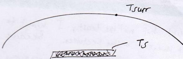
A blackbody is an idealized physical body that absorbs all incident electromagnetic radiation. Besides it is an ideal emitter. It emits much more radiation as any other body at the same temperature.
