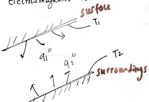
hot radiation heat exchange between two surfaces.
