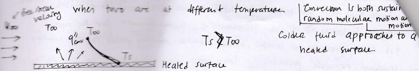
$$q''_{\text{conv}} = h [T_s - T_{\infty}] \quad (\text{Newton's law of cooling})$$
