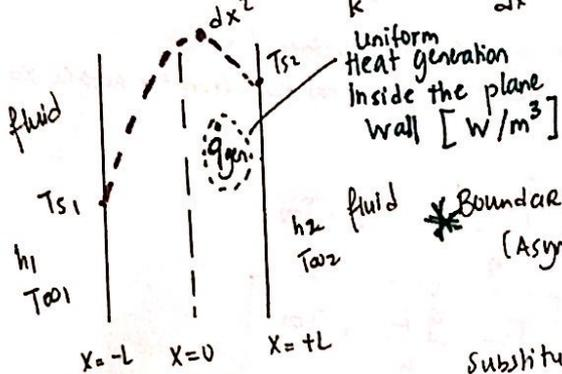
Boundary conditions  $\rightarrow$   $x = -L \quad T = T_{s1}$
