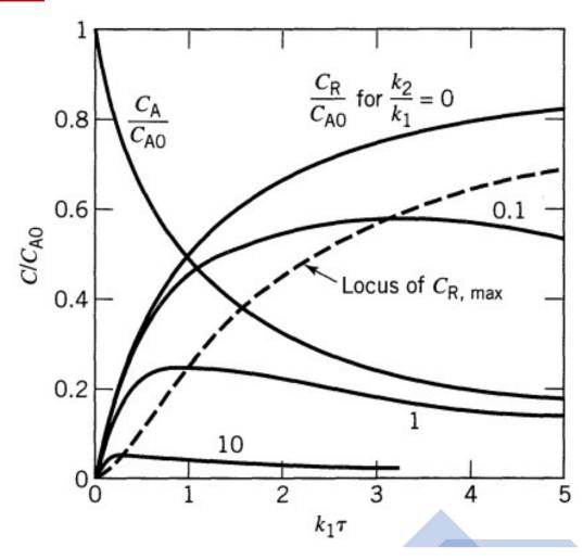
Comparison of the fractional yields of R in mixed flow and plug flow reactors for the unimolecular-type reactions
