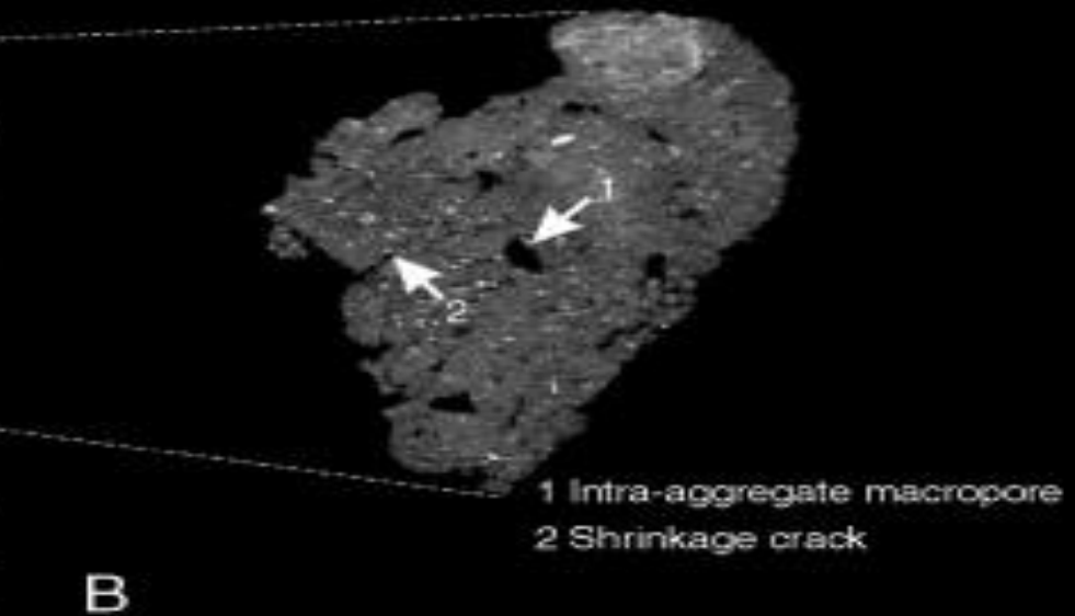
(A) A soil particle with 5mm dimension in 3D, (B) cross section view, (C-D) pore distribution
