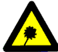
Warning laser hazard
