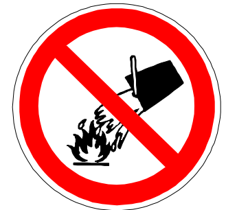
Do not extinguish with water
