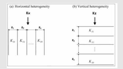
Three formations, each 25 m thick, overlie one another. If a constant-velocity flow field is set up across the set of formations with h=100 m at the top and h=80 m at the bottom, calculate h at the two internal boundaries. The hydraulic conductivity of the top formation is 0.0001 m/s, the middle formation is 0.0005 m/s, and the bottom formation is 0.001 m/s.
