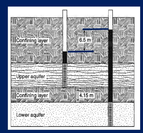
Two confined aquifers are separated by an aquitard. The hydraulic head difference between the upper and lower aquifers are 6.5 m. The vertical hydraulic conductivity of the aquitard is 0.046 m/day. What would be the leakage amount and the direction of the leakage inside the aquitard in an area of 0.5 km<sup>2</sup>. Calculate the travel time of a water molecule inside the aquitard (aquitard thickness: 4.15 m)?
