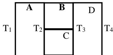
$$q = \frac{T_1 - T_4}{\frac{L_1}{k_A A_A} + \frac{1}{\frac{L_2}{k_B A_B} + \frac{1}{\frac{L_3}{k_C A_C}} + \frac{L_4}{k_D A_D}}}$$
