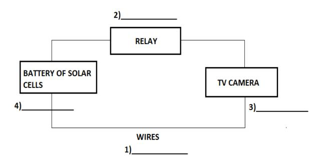
The function of this circuit is to operate a TV camera aboard a space satellite. Here the source is a battery of solar cells. A solar cell is an electric cell which converts sunlight into electrical energy. The load is the TV camera. The transmission system is the connecting wires. The control is a relay actuated by transmissions from ground control. Although the function of this circuit is much more complex than that of the flashlight, it too consists of the four basic elements.
