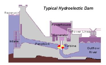
So just how do we get electricity from water? Actually, hydroelectric and coal-fired power plants produce electricity in a similar way. In both cases a power source is used to turn a propeller-like piece called a turbine, which then turns a metal shaft in an electric generator, which is the motor that produces electricity. A coal-fired power plant uses steam to turn the turbine blades; whereas a hydroelectric plant uses falling water to turn the turbine. The results are the same.
