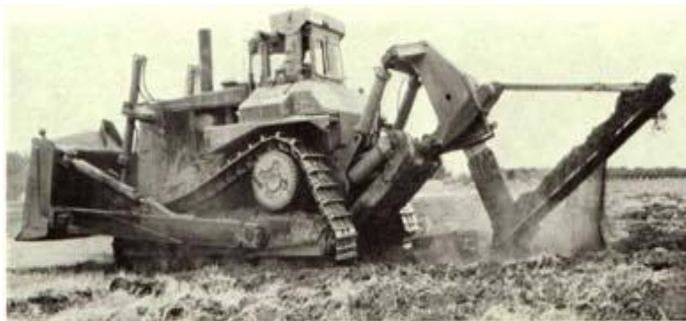
Figure 7. Slip plow; can operate six feet deep. 14 inch wide slip plate causes more heaving and displacement of layers than a ripper shank.
