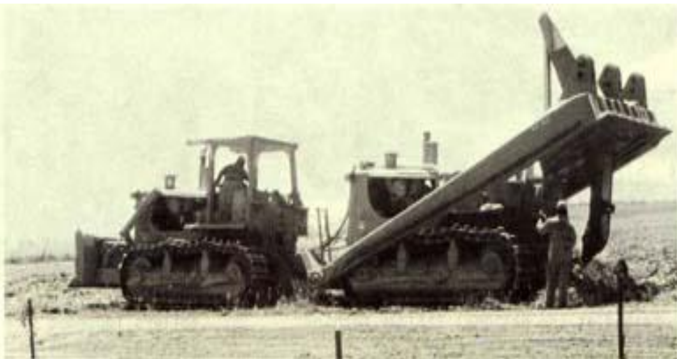
Figure 7. Slip plow; can operate six feet deep. 14 inch wide slip plate causes more heaving and displacement of layers than a ripper shank.
