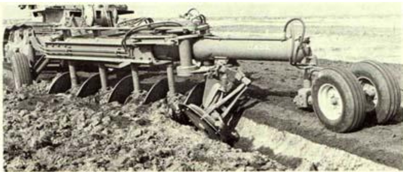
Figure 6. Disc plowing 20 inches deep. 30 inch depth attainable with larger discs. Furrow wheel enables replowing of loose soil.
