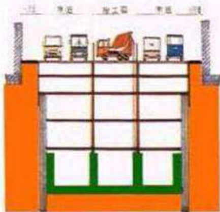
4. Construction of main structure (down - up)
