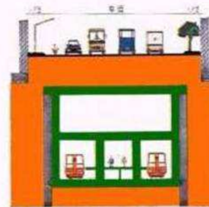
6. Completion of underground station
