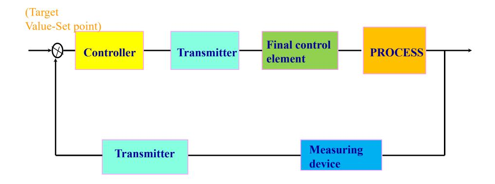
The block diagram of closed loop feed back control system
