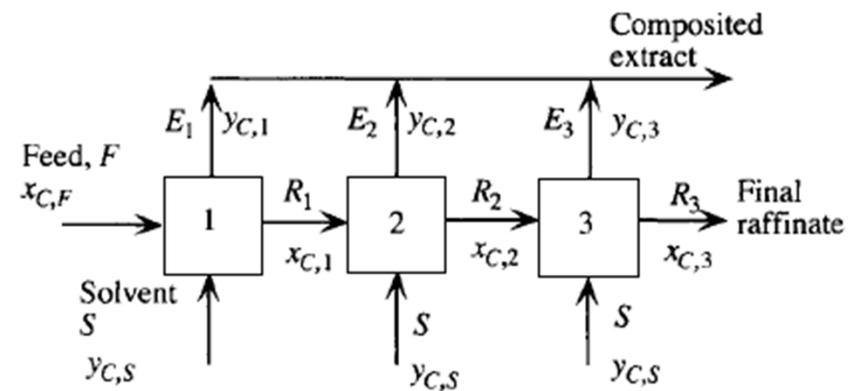
The schematic diagram for a three-stage crosscurrent extraction process
