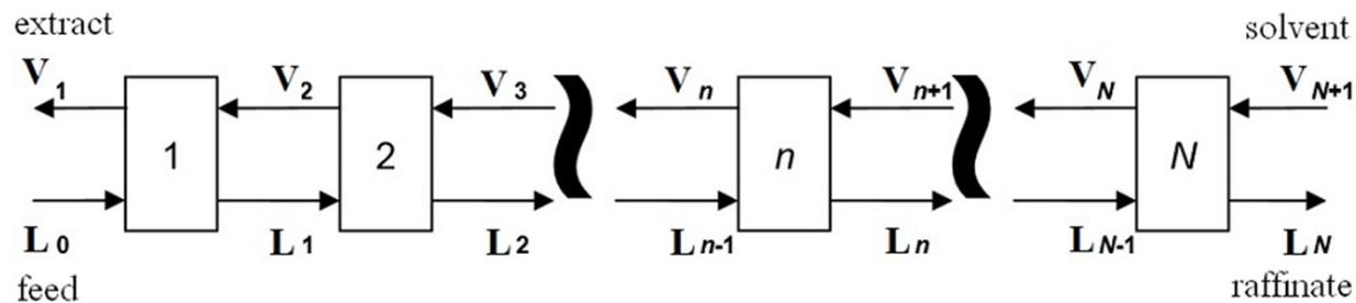
Schematic representation of a multistage countercurrent extraction process
