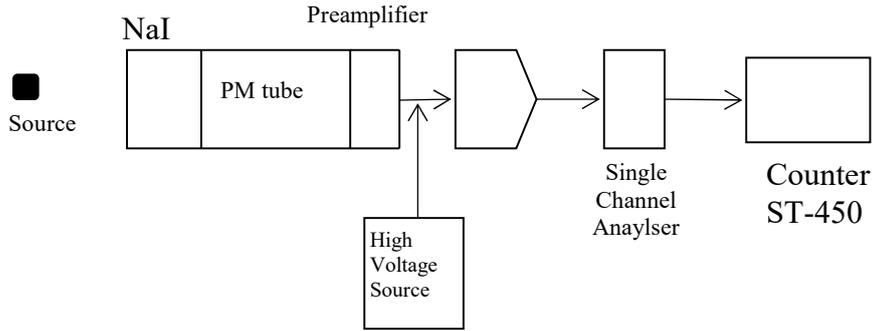
Şekil 1. The schema of NaI dedektör- ST-450 single channel analyser system
