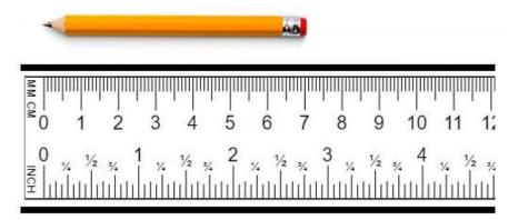
We can say that the length of the pencil is equal to 71 mm, but not 71.15 according to the ruler we used to measure the pencil.
