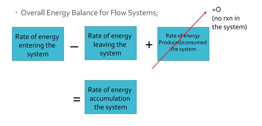
• BERNOULLI EQUATION is a particular form of a mechanical energy balance to describe the frictionless flow of an incompressible fluid along a streamline at steady state.
