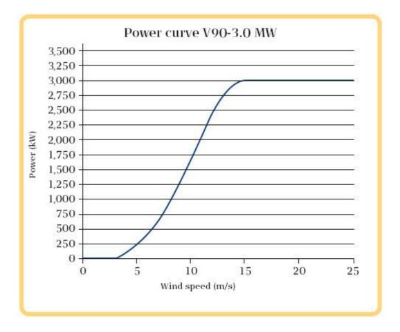
**Figure 1.** The optimal wind speeds needed to extract varying amounts of power using a Vesta V90 – 3.0 MV wind turbine.
