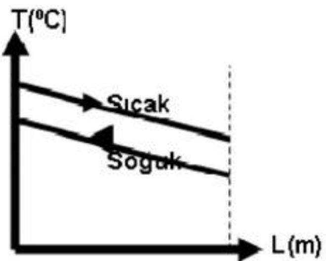
$$Q = m_h \cdot C_{Ph} \cdot \Delta T_h = m_c \cdot C_{Pc} \cdot \Delta T_c$$
