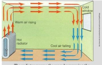
The radiator warms the room by warming the air around it. Then the warm air *transfers heat* to the rest of the room through convection.
