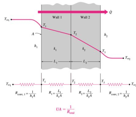
Consider a composite wall made of two different layers having different thermal conductivities. Heat transfer is at steady state and there is no generation in the system. It means heat transfer rate through different layers of wall are the same.
