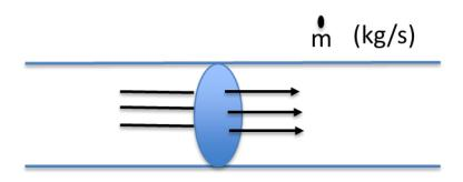
The density can be used in the conversion of volumetric flow rate to mass flow rate or vice versa.
