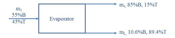
Basis: 100 kg mixture  $\Rightarrow$  m<sub>1</sub>=100 kg
