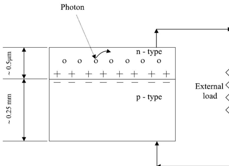
**Figure 1.** Simple PV cell and resistive load
