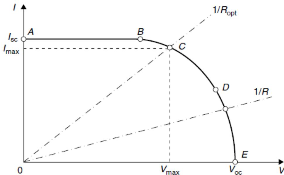
**Figure 3.** Representative current-voltage curve for photovoltaic cells.
