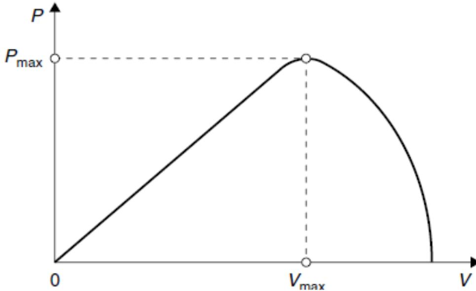
**Figure 4.** Representative power-voltage curve for photovoltaic cells.
