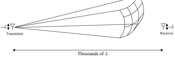
For example, a radio transmitter which broadcasts at 100MHz can reach to 40-50 km without a repeater. For such a case, assuming a receiver antenna 15 km away, the wavelength at 100MHz:
