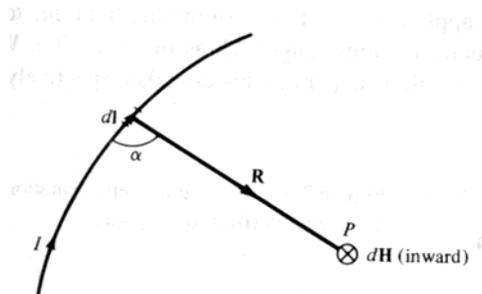
Magnetic field  $d\mathbf{H}$  at P due to current element  $I d\mathbf{l}$ .
