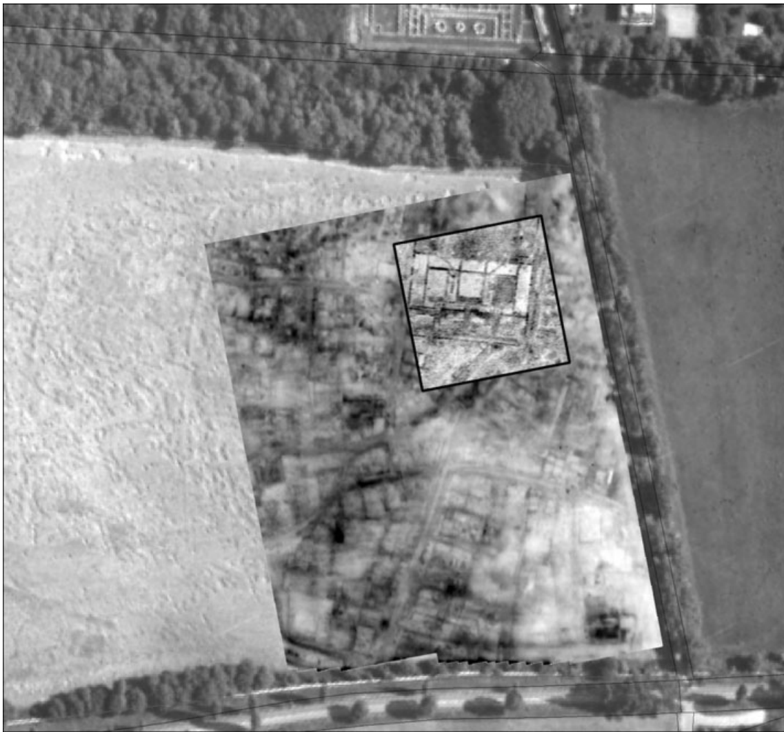
Figure 8. Orthophotograph superimposed with the result of the resistivity and the GPR survey. Resistivity: twin array, a = 0.5 m, 80\text{--}180\ \Omega\text{m} . GPR: depth slice 1.0\text{ m} - 2.0\text{ m} . Areas with high reflection energy are visualized in black. Orthophotograph release number: BMLV Nr.: 13.088/12-1.4/00.
