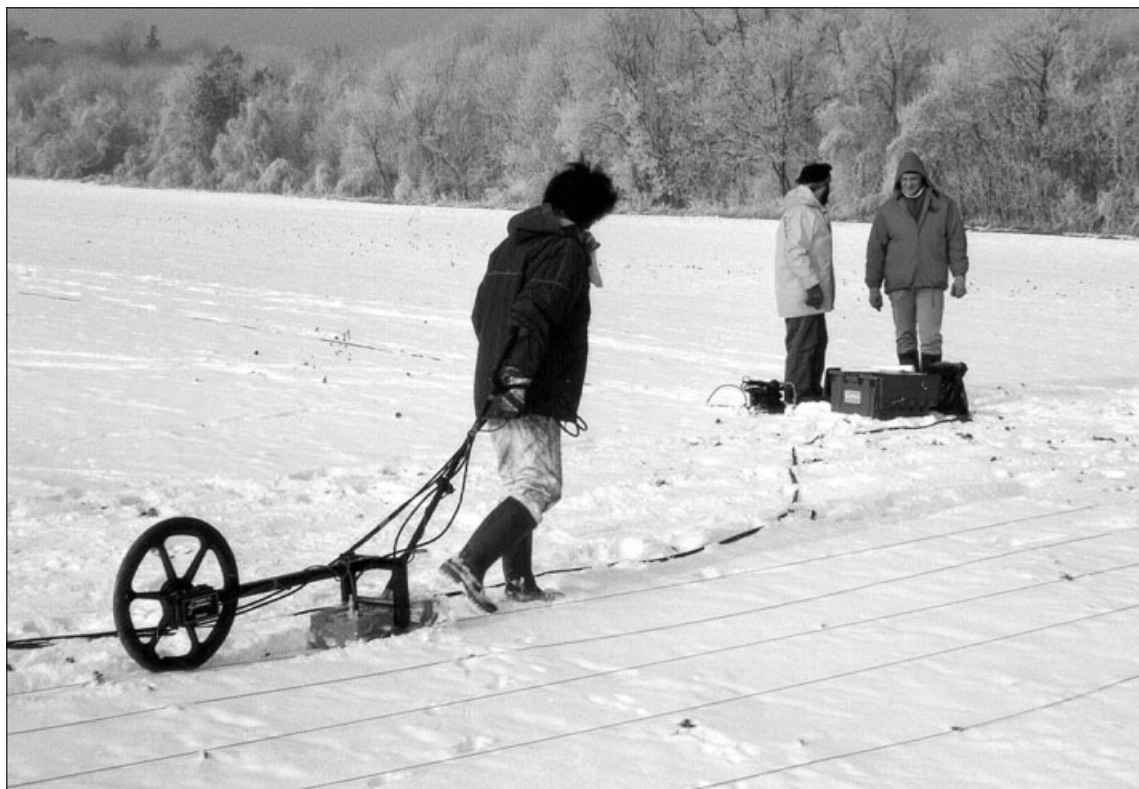
Figure 3. The GPR system PulseEKKO 1000 equipped with 450 MHz antennae and odometer during measurement at the Roman town of Carnuntum in winter 1998. The parallel measuring lines have a distance of 50 cm.
