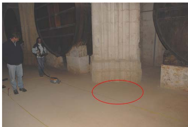
Figure 3. Ground-penetrating radar data acquisition over the Romanesque limestone pier. The red oval indicates the location of the buried pier. The floor shown in this photograph corresponds approximately to the blue rectangular region indicated in the previous figure. This figure is available in colour online at wileyonlinelibrary.com .
