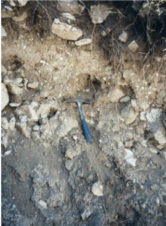
Figure 10. Sandy to silty loose soil with limestone clasts in archaeological test soundings. This corresponds to resistivity layer 2.
