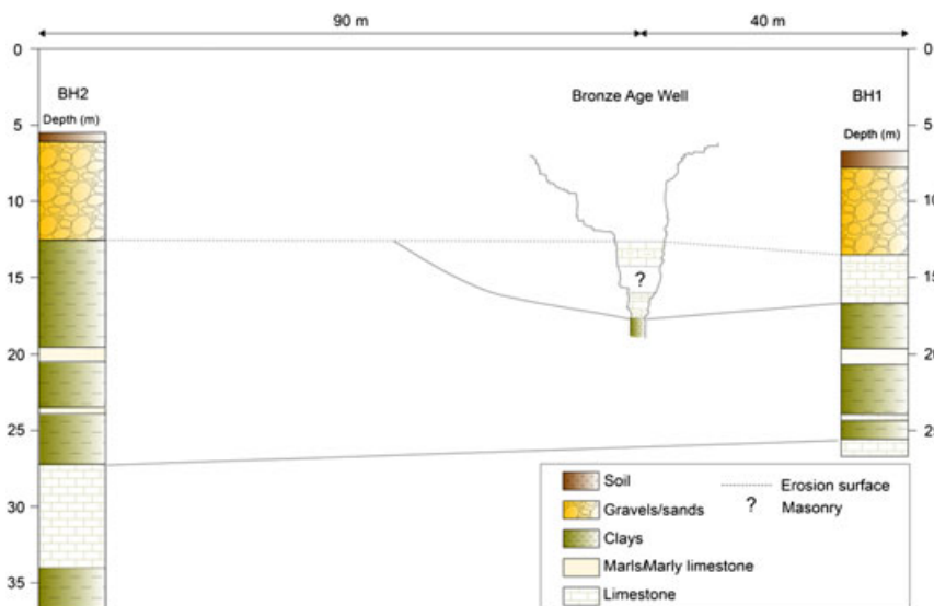
Figure 3. Lithostratigraphic correlation between the two geotechnical boreholes and the Bronze Age well (modified from EGM–GEA, 2007). Note that the horizontal scale is broken. BH1 is 40 m east, and BH2 90 m west, of the Bronze Age well. This figure is available in colour online at wileyonlinelibrary.com/journal/arp
