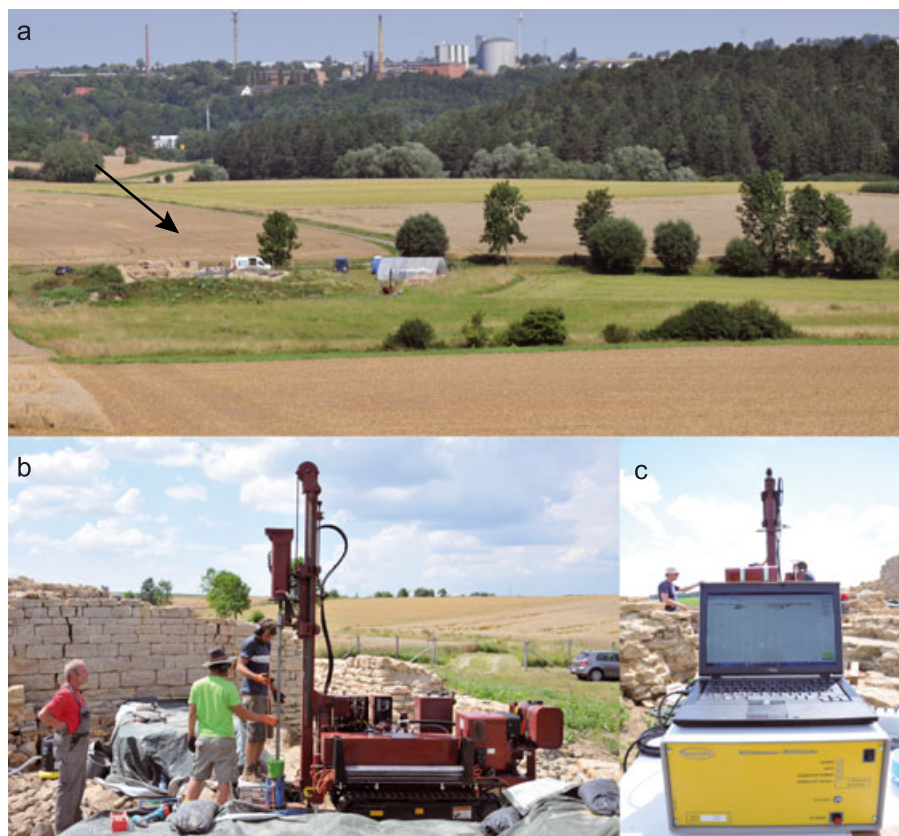
Figure 3. Excavation site of the Holsterburg lowland castle (black arrow) in the loess landscape of the Warburger Börde (a). The city of Warburg is visible in the background of the picture. Nordmeyer RS 0/2.3 drill rig with mounted Geoprobe DP-EC logging unit conducting HOL 4 within the castle (b). Geoprobe Field Instrument logging electrical conductivity and rate of penetration data as well as pushing depth (c) (photographs: A. Vött, July 2014). This figure is available in colour online at wileyonlinelibrary.com/journal/arp
