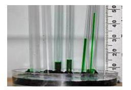
Figure : The Phenomenon of Capillary Action. Capillary action seen as water climbs to different levels in glass tubes of different diameters. Credit: Dr. Clay Robinson, PhD, West Texas A&M University.
