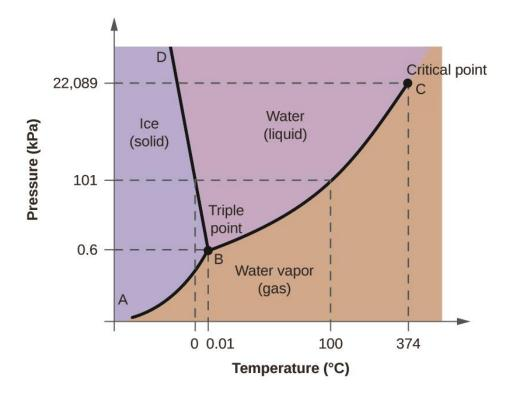
Figure : The pressure and temperature axes on this phase diagram of water are not drawn to constant scale in order to illustrate several important properties.
