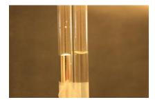
Figure: The Phenomenon of Capillary Action. Capillary action of water compared to mercury, in each case with respect to a polar surface such as glass.
