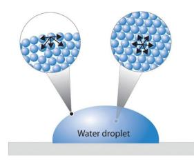
Figure: A Representation of Surface Tension in a Liquid. It presents a microscopic view of a liquid droplet.
