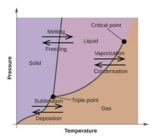
Figure : The physical state of a substance and its phase-transition temperatures are represented graphically in a phase diagram.
