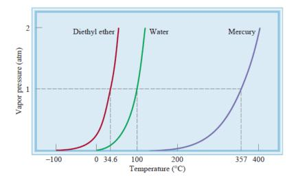
Figure. The increase in vapor pressure with temperature for three liquids. The normal boiling points of the liquids (at 1 atm) are shown on the horizontal axis.
