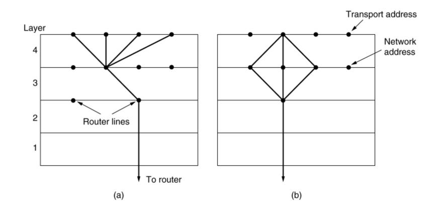
(a) Upward multiplexing. (b) Downward multiplexing.
