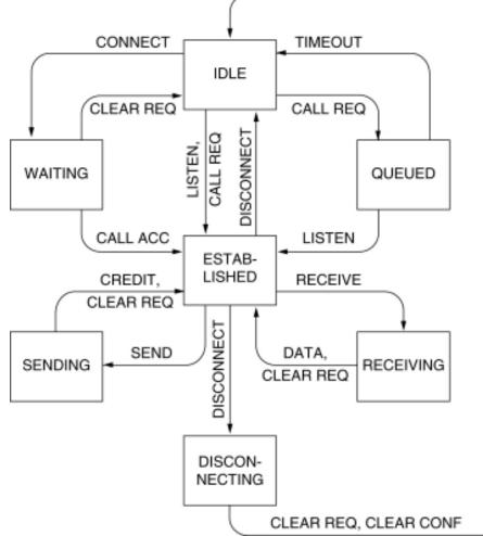
The example protocol in graphical form. Transitions that leave the connection state unchanged have been omitted for simplicity.
