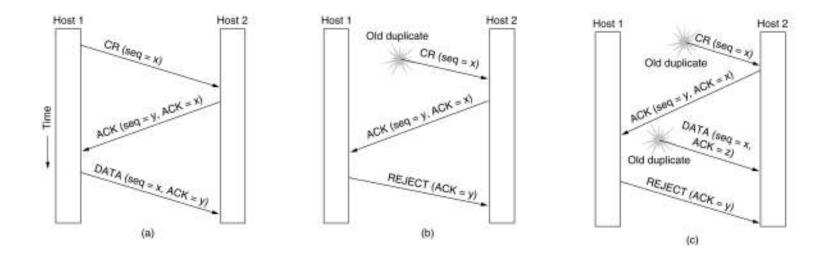
Three protocol scenarios for establishing a connection using a three-way handshake. CR denotes CONNECTION REQUEST.
