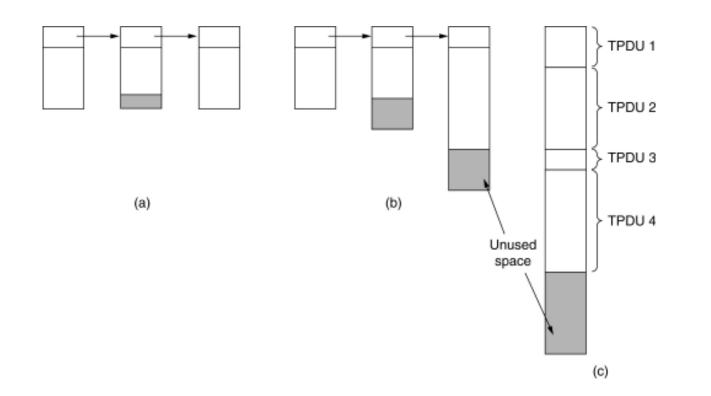
(a) Chained fixed-size buffers. (b) Chained variable-sized buffers.(c) One large circular buffer per connection.
